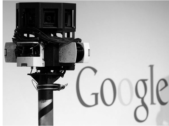
Google Street View camera/LIDAR configuration
